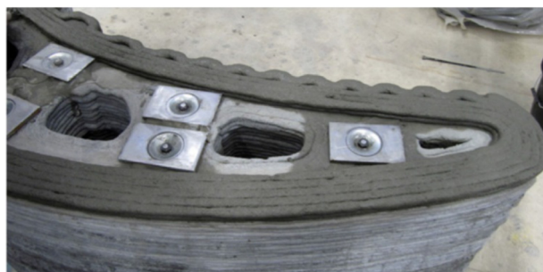
Fig. 5. Digital manufacturing of a free-shaped wall-like concrete bench using the ‘Concrete Printing’ approach [30, 31].
