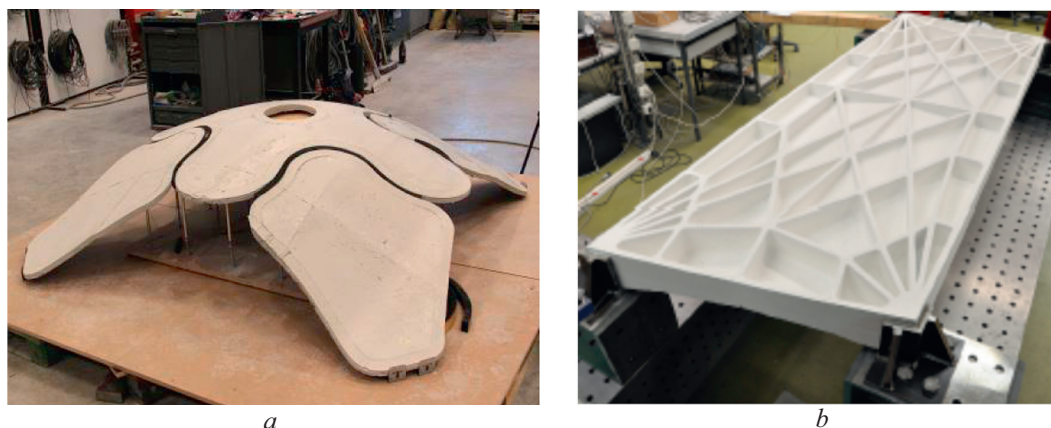
Fig. 4. Compression loaded structures: (a) self-supporting shell, constructed from double curved segments printed and cast on a flexible mould; (b) thin-vaulted, unreinforced concrete floor built with digitally fabricated formworks [29].
