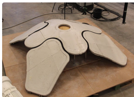
a) a panel, horizontally printed, shell and fill application. Image: 4TU project 3D printing on flexible mould TU Delft and TU Eindhoven, Netherlands.
