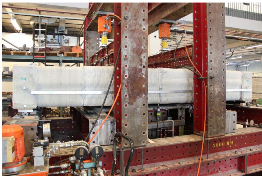
Fig. 7. 1:2 scale model of 3D concrete printed pedestrian and bicycle bridge tested in 3-point bending.
