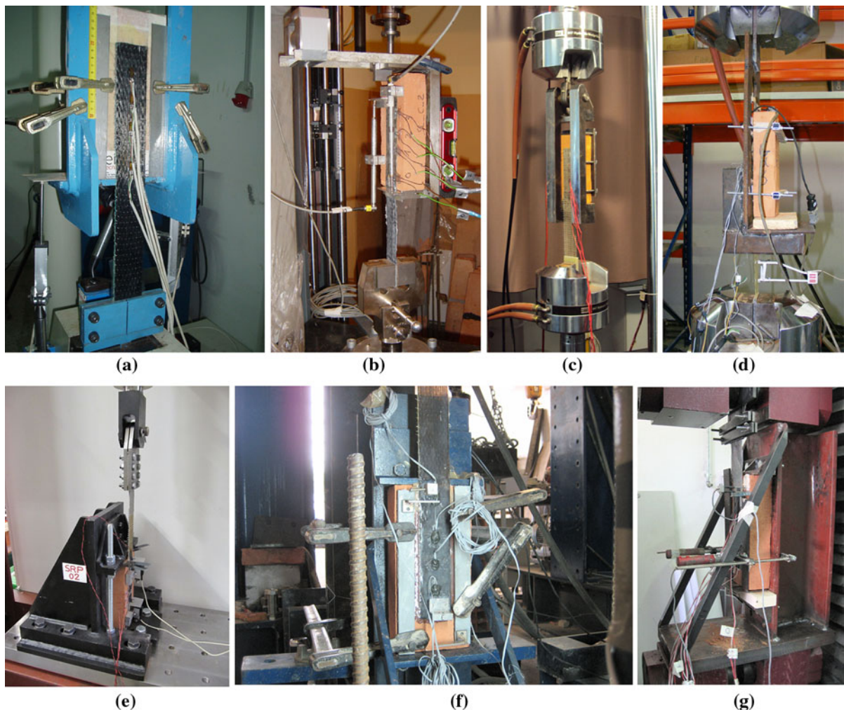
Fig. 7 Test set-ups used at TECN (a), CUT (b), UPATRAS (c), UNIRM3 (d), UNIPD (e), UMINHO (f) and UNILE (g)
