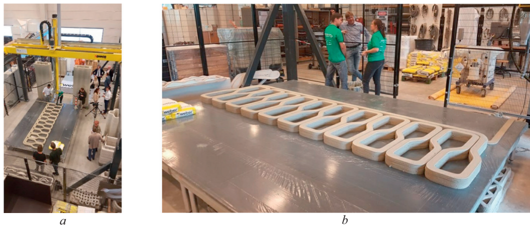
Fig. 6. Printed showcase segment for the pedestrian and bicycle bridge. The bridge consists of 6 of segments of 99 cm height that have been printed, rotated 90°, stacked together and bonded with epoxy adhesive, before being further joined by post-tensioned prestressing tendons.
