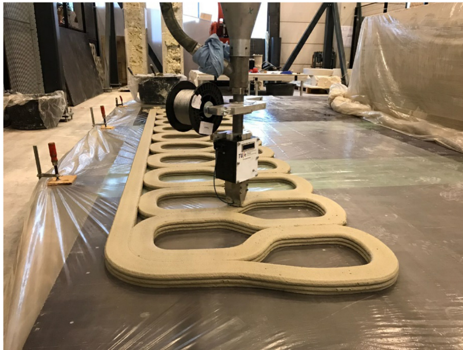
Fig. 10. Printing with the Reinforcement Entraining Device (RED) to introduce a steel cable into the concrete layer.
