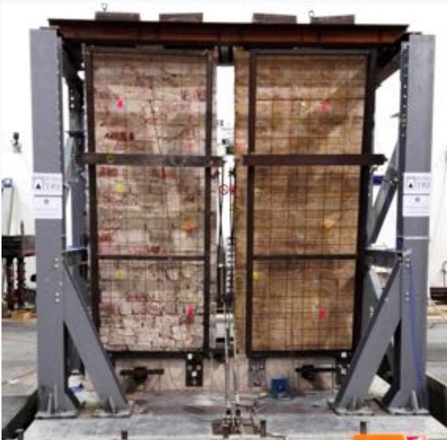
Unreinforced wall specimens on the shake table during the previous experimental investigation
