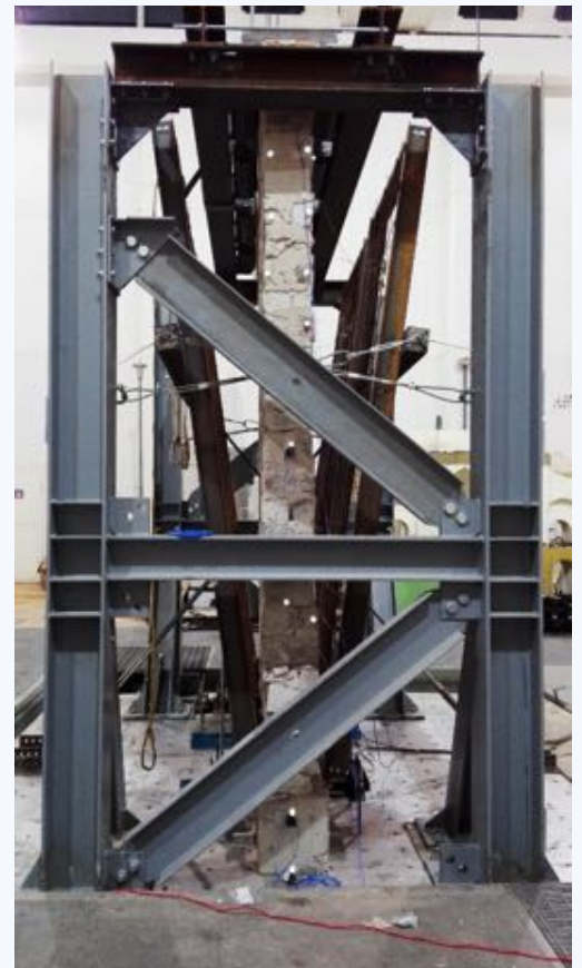
Unreinforced wall specimens on the shake table during the previous experimental investigation
