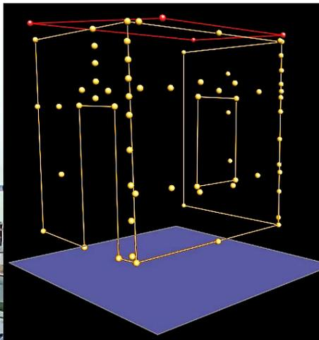
*Position of the markers on the specimen and 3DVision motion capture system for the measurement of spacial displacement in shake table tests.*
