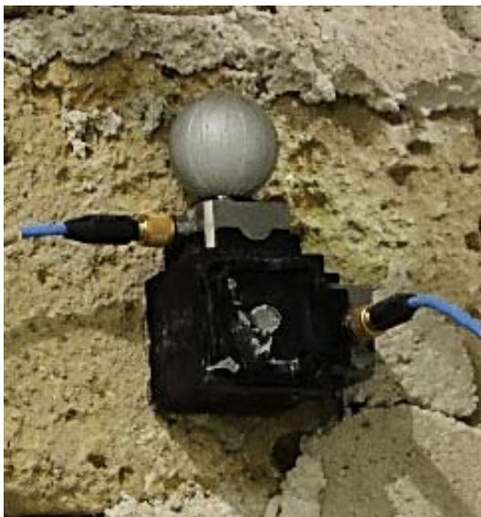
Piezoelectric accelerometer and retro-reflecting marker for 3DVision Motion Capture System
