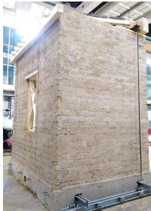
Views of the full-scale tuff masonry structure that will be tested on the shake table during the preparation of the experimental setup
