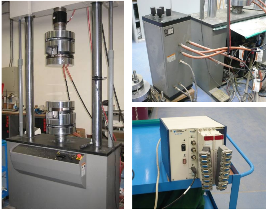
Figure 2.1. MTS testing machine (left) and detail of the oil control device (right, up) and of the data acquisition device (right, bottom).
