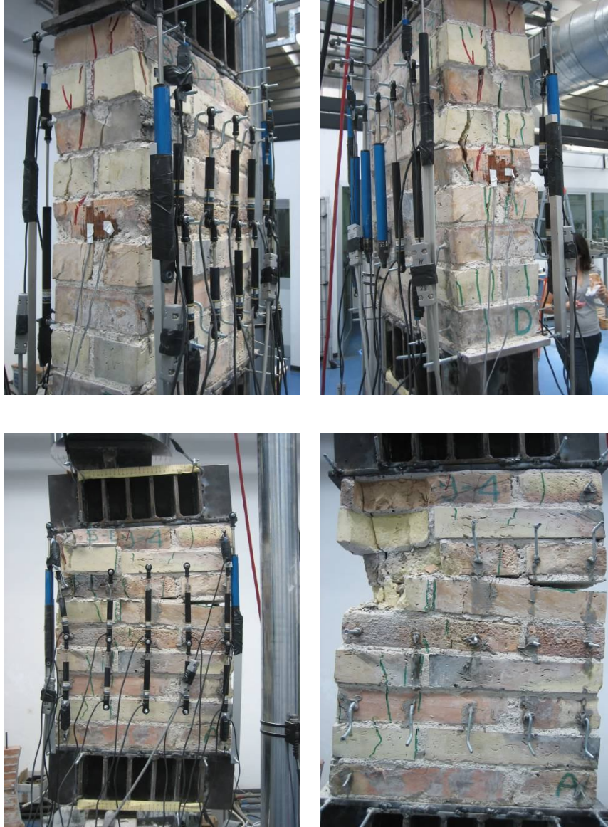
Figure 2.41. Crack pattern evolution of eccentric axial load test on S-E9-4 brickwork specimen.
