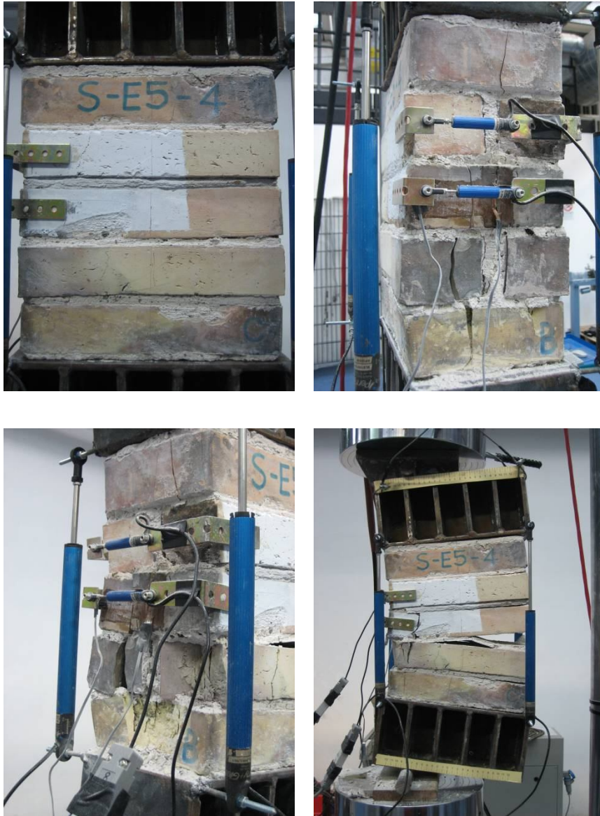
Figure 2.40. Crack pattern evolution of eccentric axial load test on S-E5-4 brickwork specimen.
