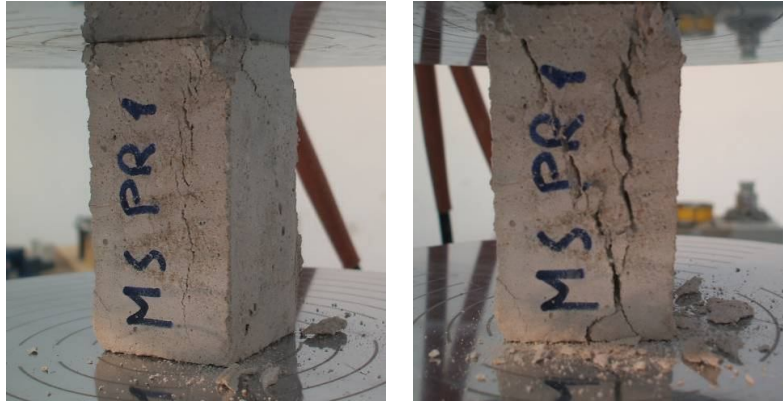
Figure 2.15. Crack pattern in a compression test on prismatic sample (slenderness ratio H/L=2 ).
