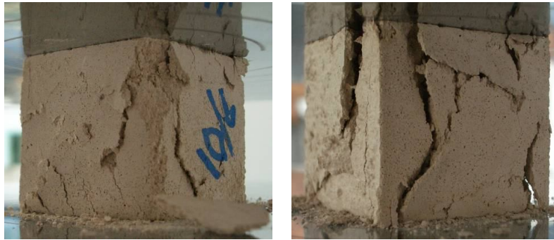
Figure 2.14. Crack pattern in a compression test on a cubic sample.
