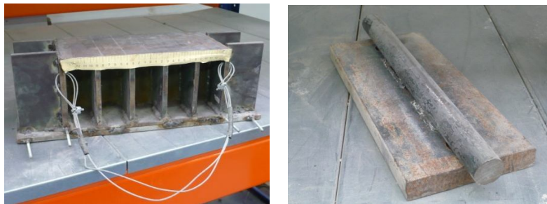
Figure 2.32. HEA-140 I-beam steel bar (left) and \varnothing 20 steel bar (right) used for eccentric axial load tests on SE-9 brickwork specimens.
