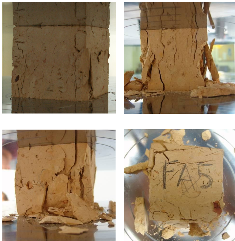
Figure 2.5. Failure pattern of an cubic brick sample during a compression test.
